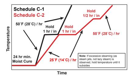
to spalls/explosions at elevated furnace temperatures. This is of special concern in floors/hearths.
